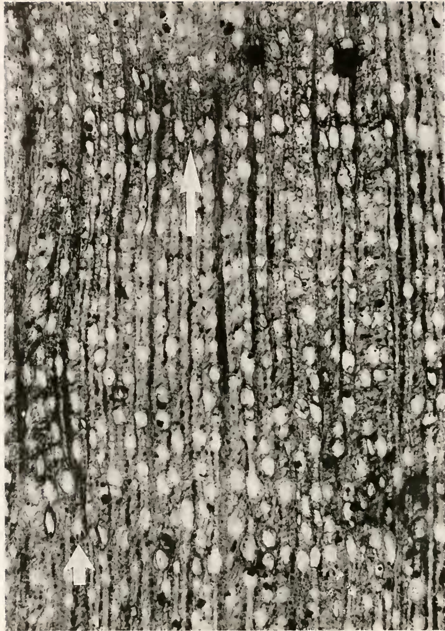
Fig. 2. Cross section (BSP 1964 I 486). Diffuse porous wood with two indistinct growth ring boundaries (arrows), uni- and multiseriate dark rays and small, oval-shaped solitary vessels; x 45
